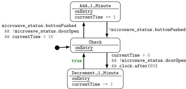
Figure 11. Simplified timer with **onEntry** sections only.
