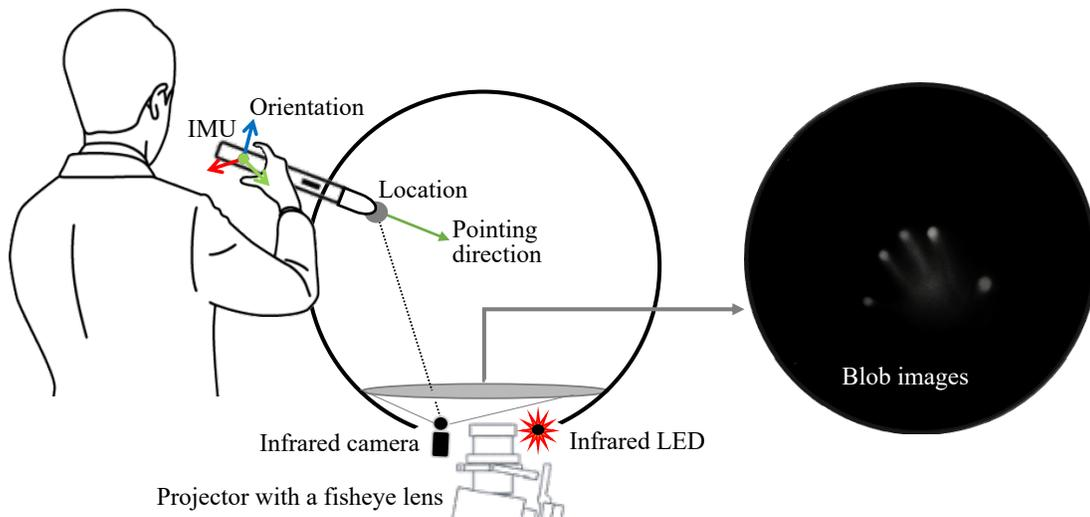
Figure 3. The mechanism of the proposed pointing device.
