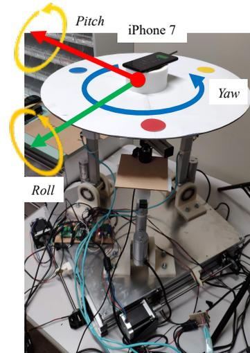
Figure 6. The Motion Platform built for this study.
