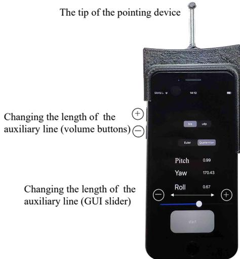
Figure 5. The proposed pointing device for the 3DSD.
