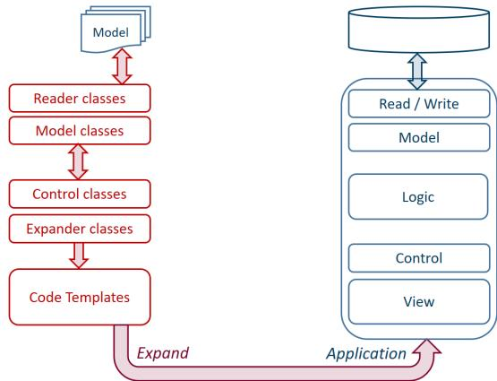
Fig. 4. Representation of a basic code generator structure.
