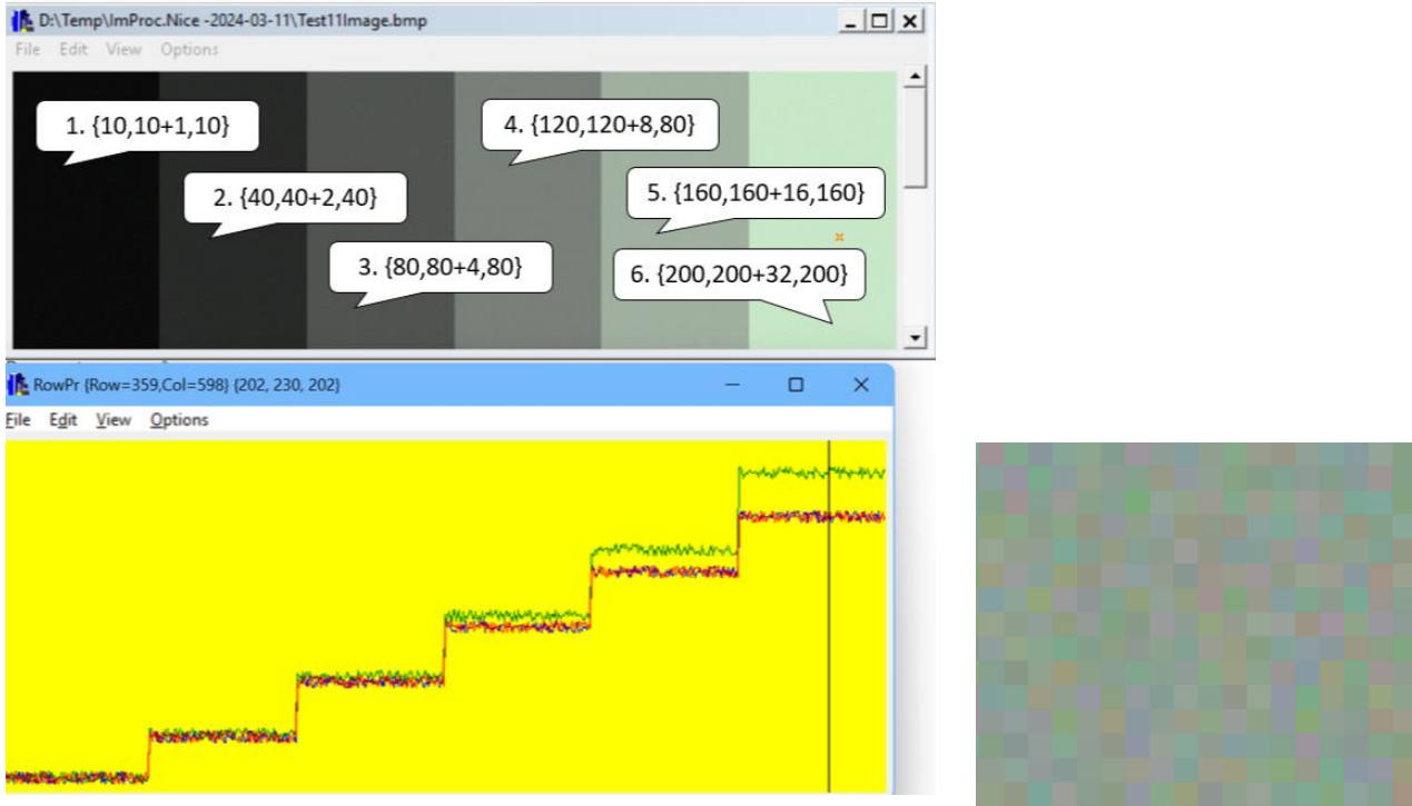
Figure 2. Upper Left: Synthetic image – 6 strips, having mix of GRAY + GREEN colors. (see callouts). Pseudo-random noise is added. Lower left: Profile of a row = 359. Specific values of the pixel of cursor are {R=202, G= 230, B = 202}, and because of noise values are slightly differ from declared values {R=200, G=232, B=200}. Lower right: scaled UP fragment from the strip #2. Saturation and brightness were set to maximum to emphasize that because of noise, nearly gray pixels (with some green tint) now have pseudorandom colors (red, green, blue, etc.).
