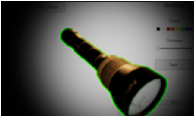
Figure 10. Screenshot, the torch with treatments: navigation, zoom, high static light and edge computed from depth gradient.
