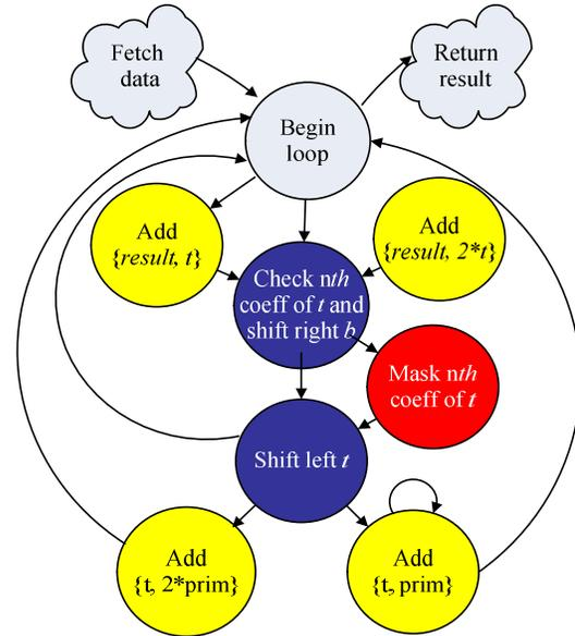
Figure 2: Arithmetic Control Unit
