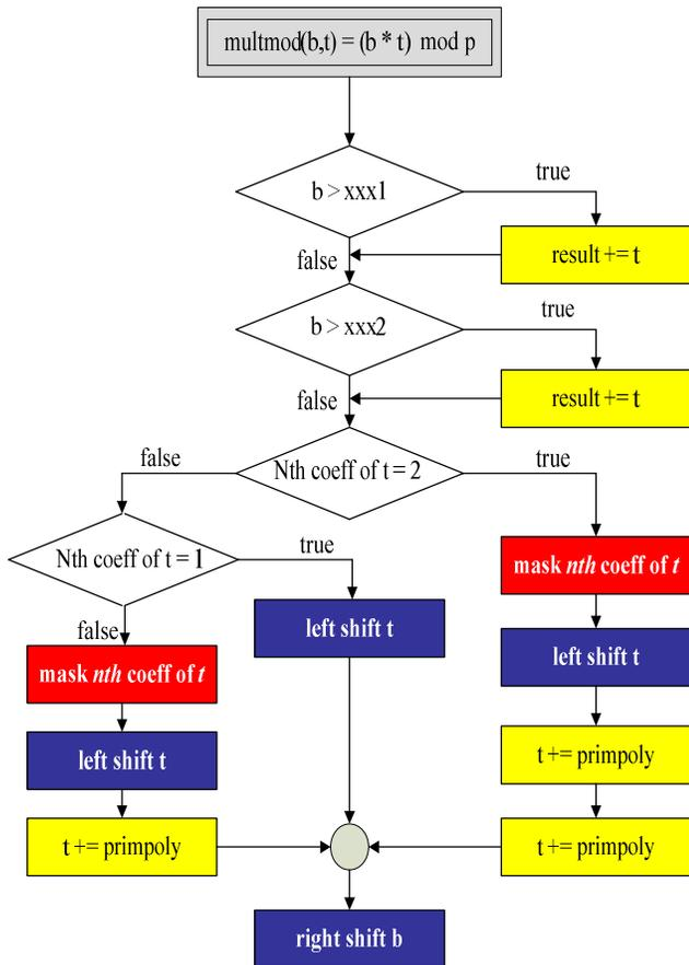
Figure 1: Arithmetic Computation Unit
