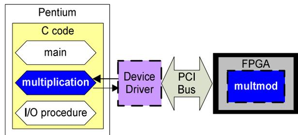
Figure 3: Overview of loosely coupled system
