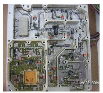
Figure 2. Uncovered on-board transceiver EM
