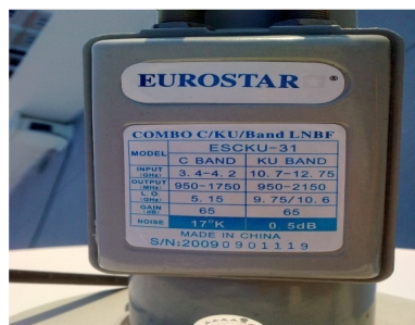
Figure 4: LNB selected in the AUS Student Satellite receiving station.
