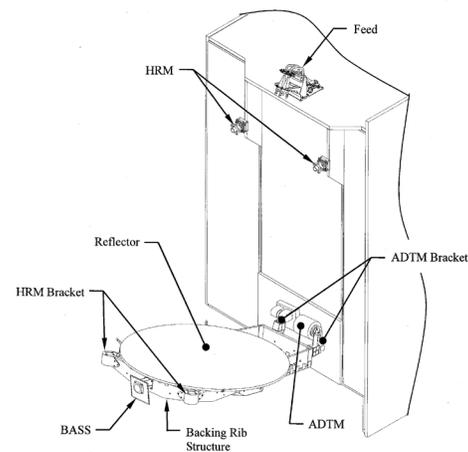
Figure 2. Illustration of Antenna Configuration (East Panel)
