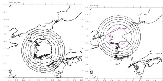
Figure 1. COMS service coverage for SK and NK beams
