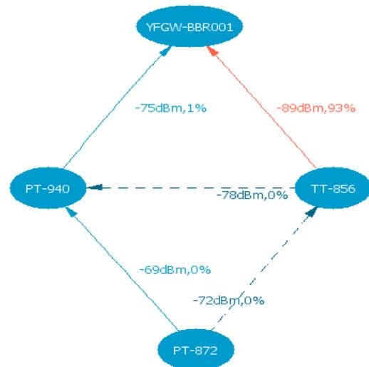
Figure 4. ISA100 test for irregular surface.
