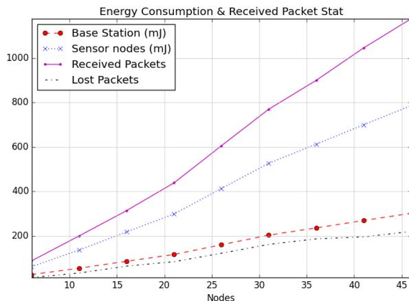
Figure 7. Energy consumption and stats at base station.
