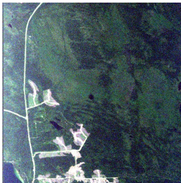
Figure 6. Linear stretched RGB radiance image simulated by MCScene for a subset of the Boreal scene for solar zenith angles of 90 degrees and a visibility of 23 km.
