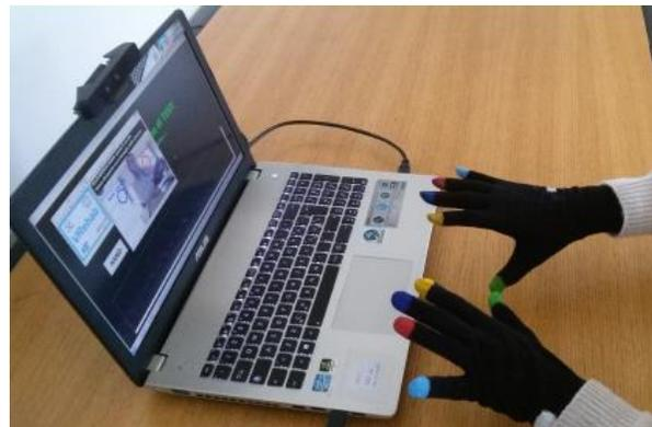
Figure 1. Hand/fingers tracking system
