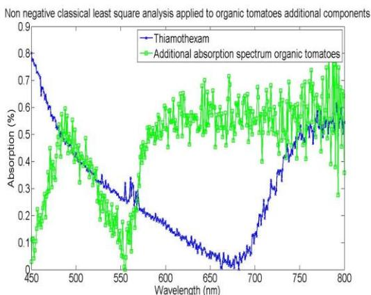
Figure 12. Organic tomatoes additional artificial components spectrum reconstructed from Non Negative Classical Least Squares analysis using the pesticides Dicofol, Thiamethoxam and Malathion spectra.
