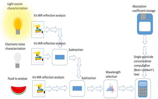
Figure 4. Food analysis procedure using the Vis-NIR reflected spectrum and the Beer-Lambert’s concentration law
