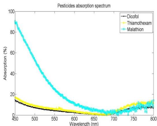
Figure 11. Vis-NIR absorption spectra of the Dicofol (concentration: 0.75e-3 Mole/L), Thiamethoxam (concentration: 0.36e-3 Mole/L) and Malathion (concentration: 1.9e-3 Mole/L).
