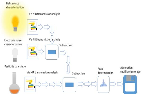
Figure 3. Pesticide absorption coefficient determination procedure
