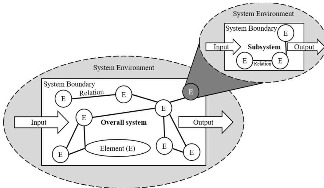
Figure 3: Structural modeling of a production system [12].
