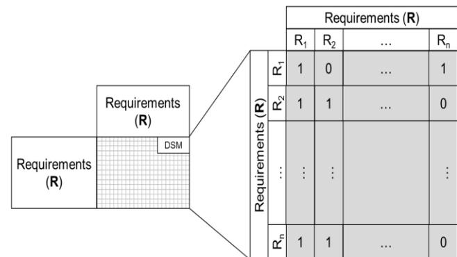
Figure 7: The DSM Matrix (Requirements View) [27].
