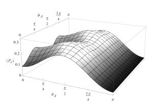
Figure 10. Error probability  $\langle P_e \rangle$  depending on  $\theta_A$  and  $\phi_A$ . Here, a standard deviation ( $\delta \varphi$ ) =  $\pi/10$  of the angles is taken into account.
