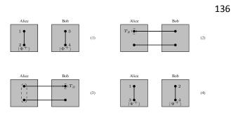
Figure 2. Sketch of a standard setup for an entanglement swapping based QKD protocol. Qubits 2 and 3 are exchanged (cf. picture (2)) and a basis transformation  $T_x$  is applied on qubit 1 and inverted by using  $T_x$  on qubit 2.
