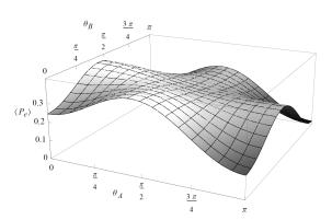
Figure 11. Error probability  $\langle P_e \rangle$  depending on  $\theta_A$  and  $\theta_B$ . The remaining parameters  $\phi_A$  and  $\phi_B$  are fixed at  $\pi/4$ . Here, a standard deviation  $(\delta \varphi) = \pi/20$  of the angles is taken into account.
