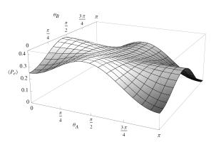
Figure 7. Error probability  $\langle P_e \rangle$  depending on  $\theta_A$  and  $\theta_B$ . The remaining parameters  $\phi_A$  and  $\phi_B$  are fixed at  $\pi/4$ .
