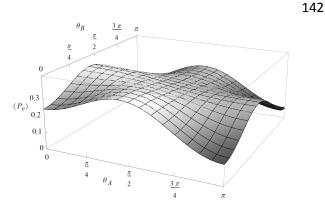
Figure 12. Error probability  $\langle P_e \rangle$  depending on  $\theta_A$  and  $\theta_B$ . The remaining parameters  $\phi_A$  and  $\phi_B$  are fixed at  $\pi/4$ . Here, a standard deviation  $(\delta \varphi) = \pi/10$  of the angles is taken into account.
