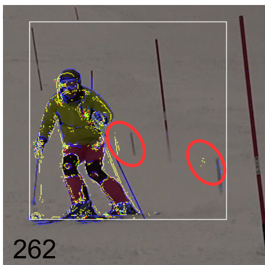
Figure 13. Frame with low shape accuracy for Skier 2. Un-eliminated background feature points (circles with red) affected the shape and tracking accuracy.
