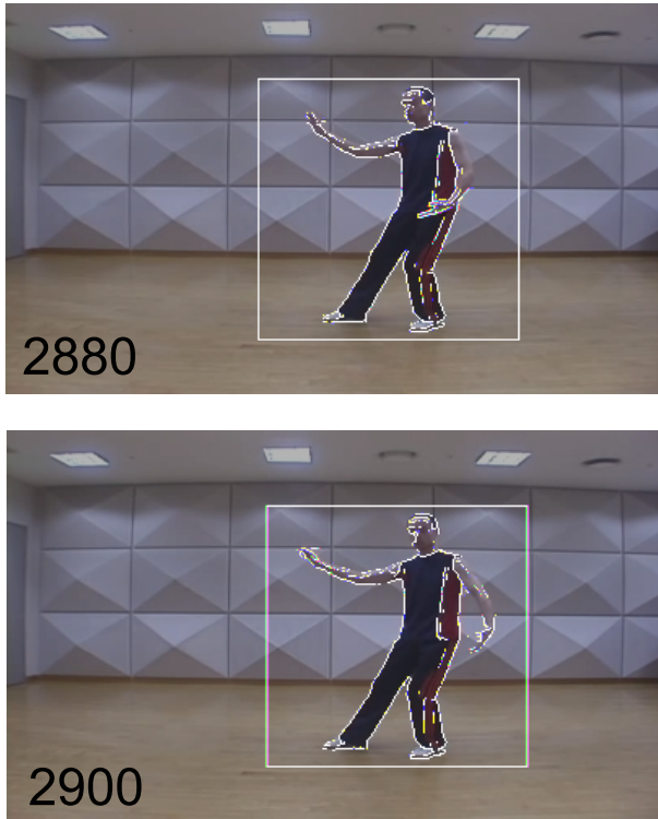
Figure 5. Tracking and shape prediction for Tai chi chuan. Blue: Ground Truth; Green: Linear Prediction; Red: Second-order Prediction.
