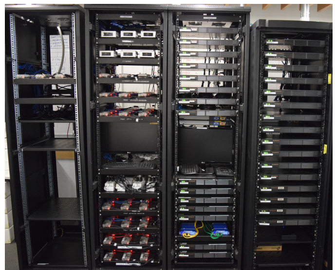
Figure 11. The Auckland Satellite TCP/IP Traffic Simulator at the University of Auckland. The two racks on the left contain the “island” machines, the next rack to the right accommodates (from bottom) capture servers, copper taps, the satellite chain, and “world” servers on the top. The rack on the right holds the remaining “world” servers, a spare, and a special purpose server.
