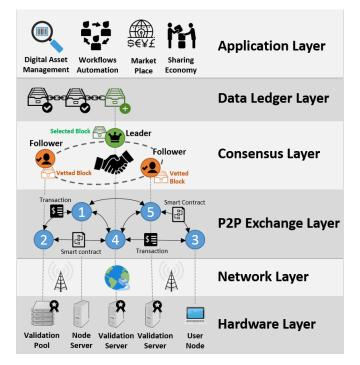
Figure 1. Blockchain High Level Architecture
