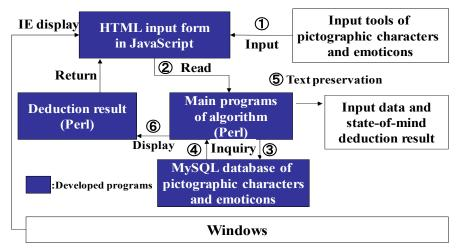
Figure 6. Block diagram of the system and programs developed
