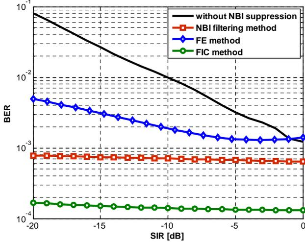
Figure 6. BER as a function of SIR for CM1 channel
