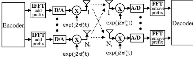
Figure 1. MIMO MB-OFDM UWB system.
