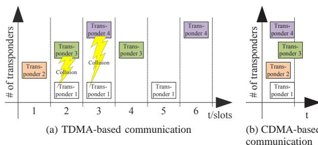
Figure 1. Different communication channel access techniques for RFID: TDMA, CDMA
