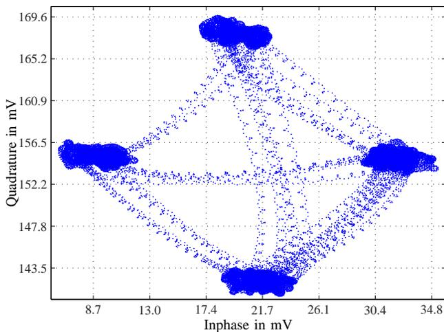
Figure 18. IQ constellation diagram for 2 transponders
