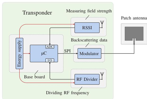
Figure 8. Block diagram of semi-passive UHF RFID transponder with limited downlink capabilities
