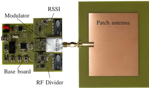
Figure 9. Prototype of semi-passive UHF RFID transponder
