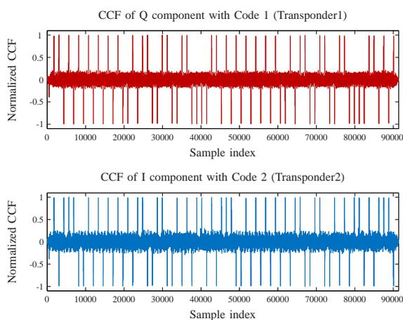
Figure 22. Cross-correlation of signals with origin spreading codes - Process of despreading / 2 Transponders
