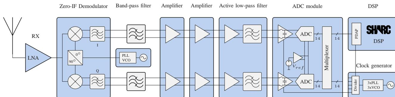
Figure 15. Architecture of receiving system
