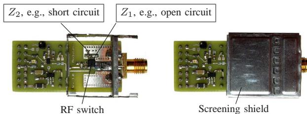
Figure 10. Backscatter modulator
