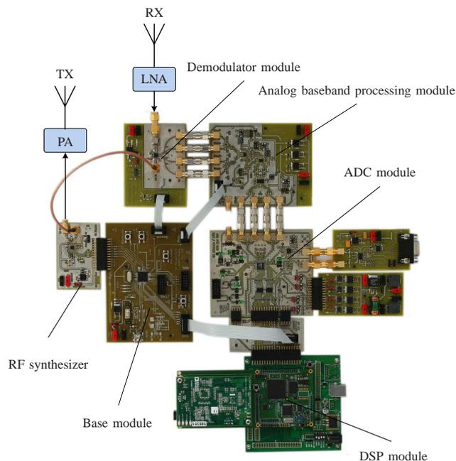
Figure 5. Architecture of CDMA-based RFID reader
