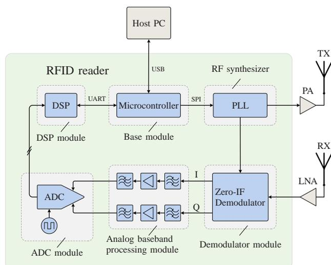
Figure 4. Basic concept of RFID reader
