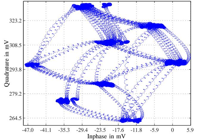
Figure 19. IQ constellation diagram for 3 transponders
