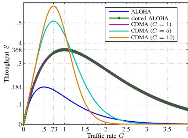
Figure 2. Various throughputs  $S$  over traffic rate  $G$  for ALOHA, slotted ALOHA and CDMA
