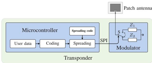
Figure 7. Concept of CDMA-based semi-passive UHF RFID transponder
