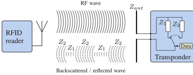
Figure 6. Basic function of RFID transponder
