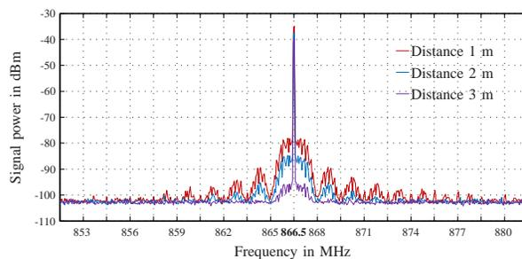
Figure 16. Spectrum of backscattered signal from transponder
