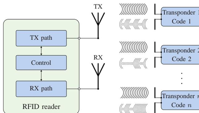
Figure 3. Basic architecture of RFID system
