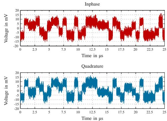
Figure 20. IQ signal after demodulator / 2 Transponders
