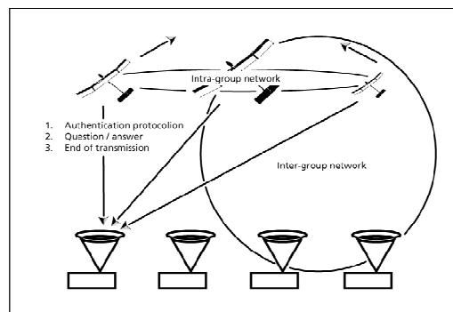
Figure 4. The principle of the network topology.
