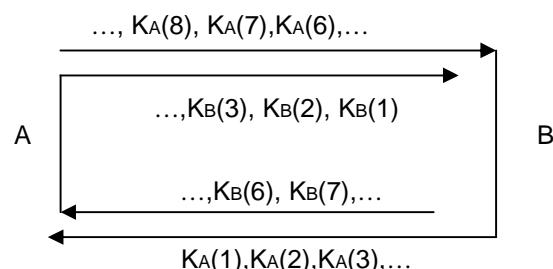
Figure 9. The basic idea of OTP exchange.
