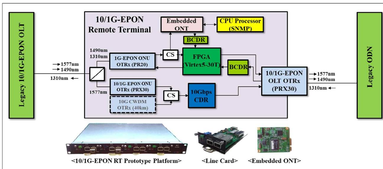
Figure 3. The design architecture and prototype of the proposed 10/1G-EPON RT.
