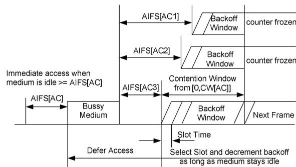
Figure 2. IEEE 802.11e EDCA mechanism [6].
