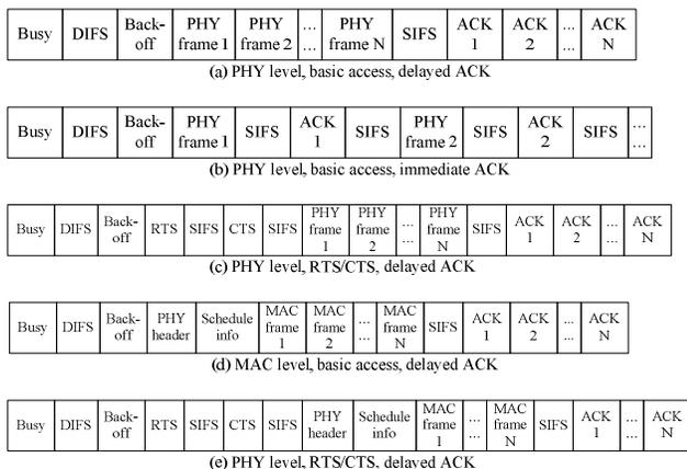
Figure 3. IEEE 802.11n Frame aggregation mechanisms [6].
