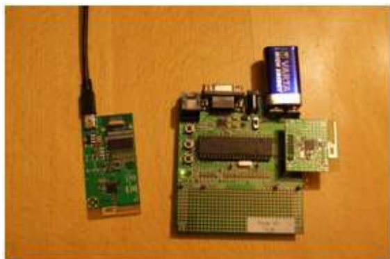
Figure 11. MicroChip sniffer (left), PICDEM Z (left).
