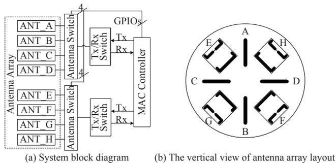
Fig. 1. The architecture of smart antenna system
