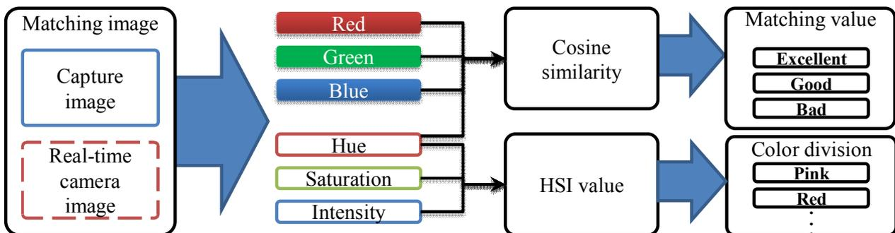
Figure 4. The flow of the color-matching algorithm
