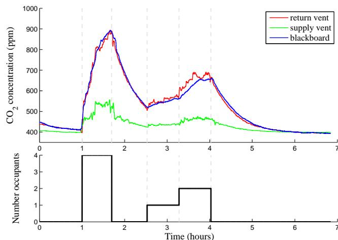
Figure 5. Occupants experiment F. Field measurements during project discussion. Top: Proxy measurements. Bottom: Corresponding occupancy.
