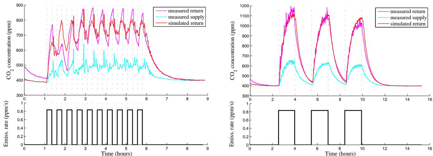
Figure 7. Proxy model simulation with CO<sub>2</sub> pump experiment A with 30 minutes (left) and experiment B with 1 hour (right) periodic excitation. Measurements at supply (green), return (blue), and simulated return (red) vents are shown.
