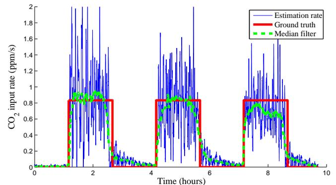
Figure 10. Sensing the latent CO<sub>2</sub> emission rate by proxy for CO<sub>2</sub> pump experiment A (left) and experiment C (right). The estimated emission rate (blue), median filtered rate (green), and ground truth (red) are given.
