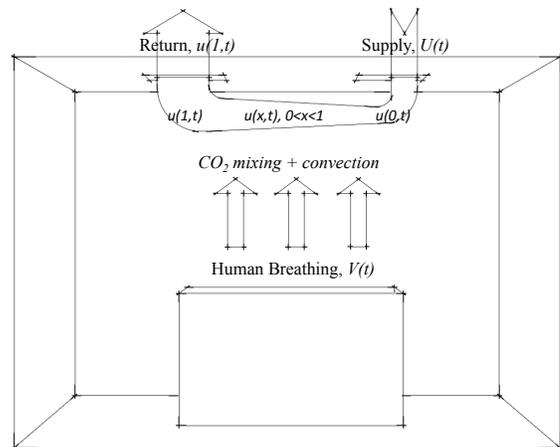
Figure 1. The physical representation of the model. Fresh air with CO<sub>2</sub> concentration  $U(t)$  enters the room from the supply vent, and exits the room after convection and mixing with human breath,  $V(t)$ , which rises to the ceilings, and the measured CO<sub>2</sub> concentration at the return vent is  $u(1, t)$ .
