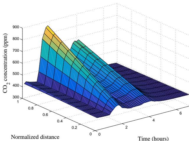
Figure 9. Spatial and temporal dynamics of CO<sub>2</sub> concentration as represented as the states in the proxy link model.
