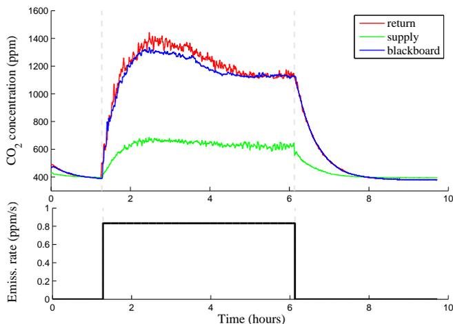
Figure 3. CO<sub>2</sub> pump experiment D. The measured CO<sub>2</sub> concentration from different locations for a 5-hour CO<sub>2</sub> release are shown.
