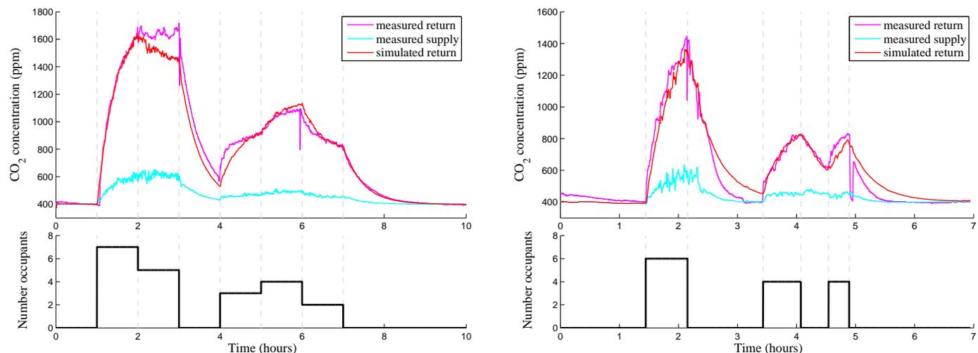
Figure 8. Proxy link model simulation with occupants experiment E (left) and G (right). The proxy measurements at return (blue), supply (green), and simulated return (red) vents are demonstrated.
