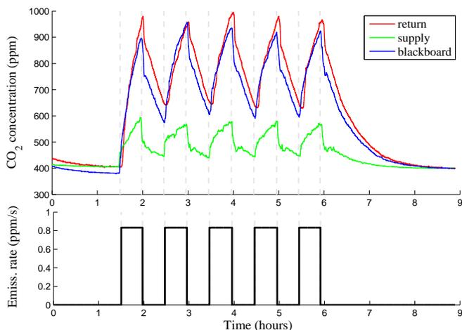
Figure 4. CO<sub>2</sub> pump experiment B. Short term excitation with period of 1 hour. Measurements at return (red), supply (green) vents, and blackboard (blue) are shown.
