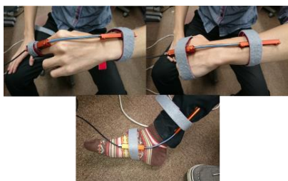
Figure 4. Mounting situation of angle sensor TMI-160
