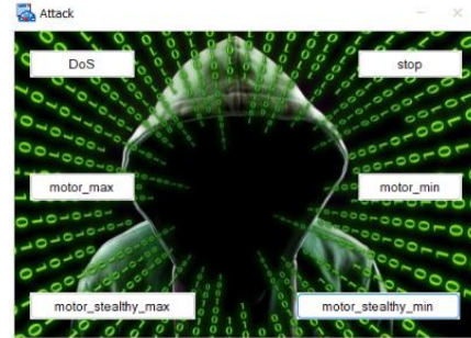
Figure 15. Panel for controlling the CAN bus attacks
