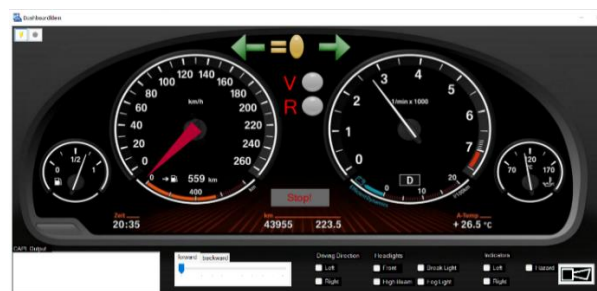
Figure 13. Dashboard for controlling the CAN bus demonstrator
