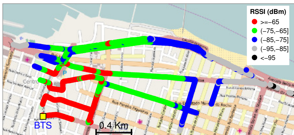
Fig. 2. Drive test with measurements in an urban area in the city of Fortaleza. The colors indicate the radio signal strength indicator (RSSI) in dBm and the yellow square represents the location of the base station (BTS).
