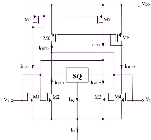
Figure 5. Negative resistance active resistor circuit
