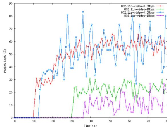
Figure 12. Packet lost comparison of 802.11e and 802.11n.
