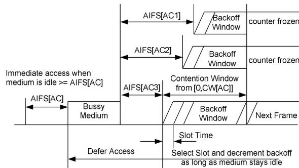
Figure 2. IEEE 802.11e EDCA mechanism [6].
