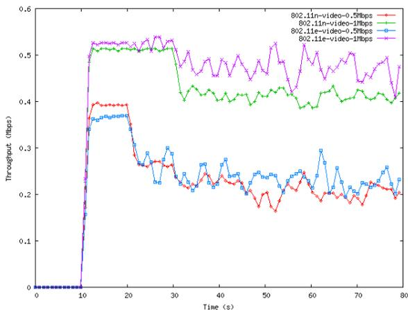
Figure 10. Throughput comparison of 802.11e and 802.11n.
