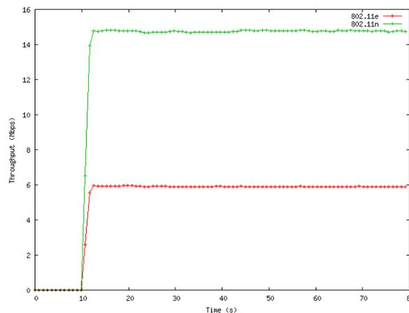
Figure 13. Maximum throughput comparison of 802.11e and 802.11n.
