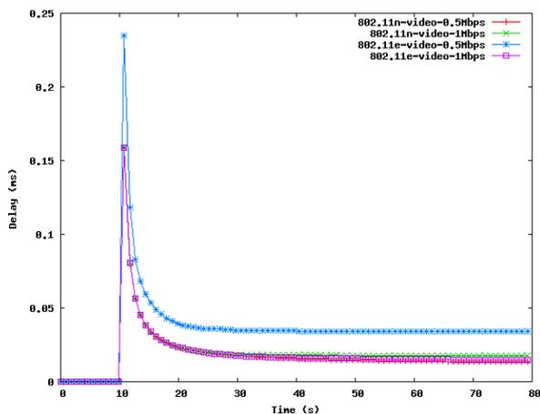
Figure 11. Delay comparison of 802.11e and 802.11n
