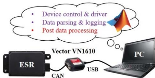
Figure 5. Radar measurement set-up.
