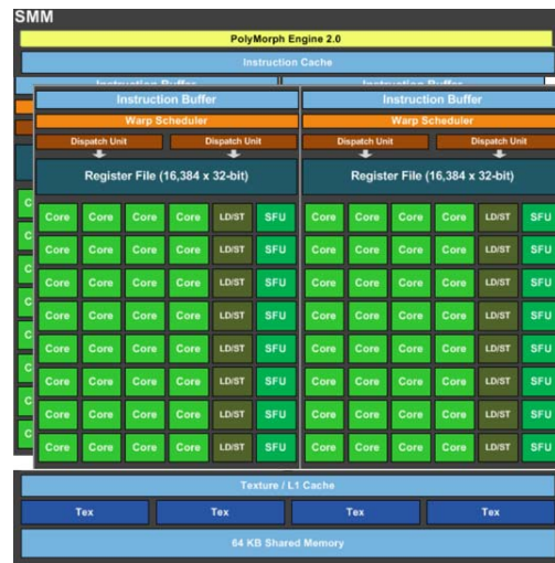
Figure 3. Maxwell Streaming Multiprocessor (SMM) block diagram. (excerpted from [6]).
