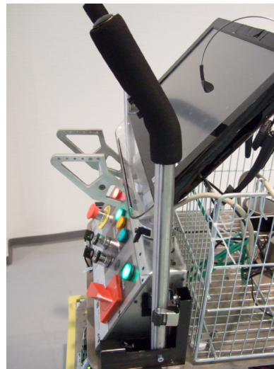
Figure 2. Implementation of the walking aid — locked position.
