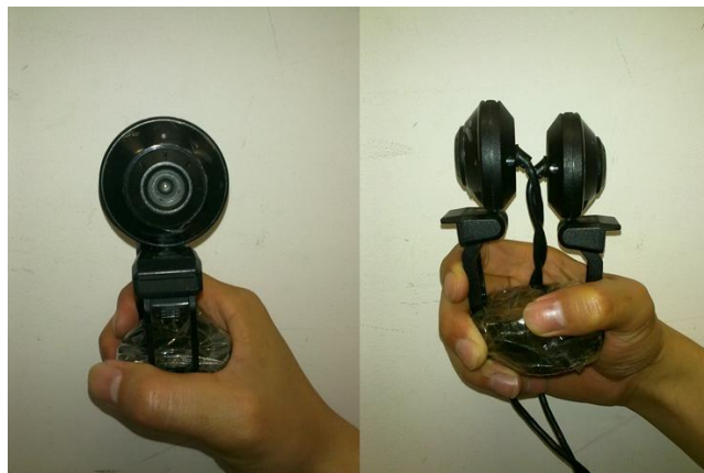
Figure 1. The Prototype of Back-to-Back. It consists of back-to-back cameras. Their unique geometric relationship is the key point we utilize.
