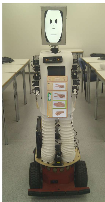
Figure 1. CHARLY (Companion Humanoid Autonomous Robot for Living with You) with 'retro robot' body covers and LCD face display showing a simple cartoon-like face.
