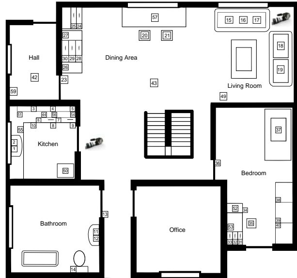
Figure 1. The UH Robot House layout and sensor arrangement. 59 sensors are available in the house, but only 52 were used and shown here. The two cameras' locations during the experiments are represented in this picture.
