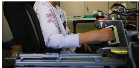
Figure 3. Handreha : The developed desktop hand rehabilitation device
