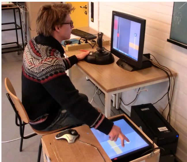
Figure 3. The “deported view” experimental setup, with the operator using a second finger to perform a click.
