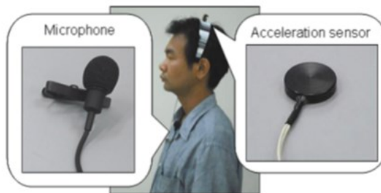
Figure 7. Acceleration sensor and microphone.
