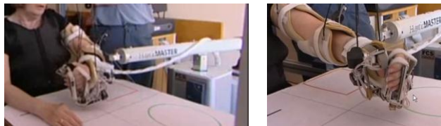
Figure 5. The Gentle/G system during a rehabilitation exercise
