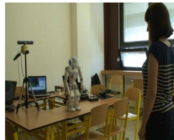
Figure 3 - Demo setup with participant, Nao robot and Kinect Device (a second Kinect device was also employed for finger detection but not used within the demos)
