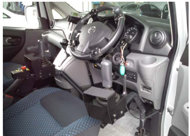
Figure 2. Wada and Kameda’s joystick driving interface
