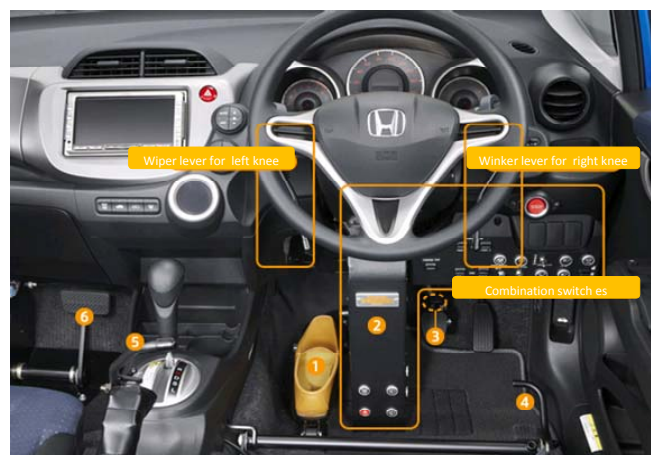
(1) Steering pedal (4) Selection bar for feet (2) Steering box (5) Side brake for knee (3) Brake lock button (6) Sub-brake for exercise
