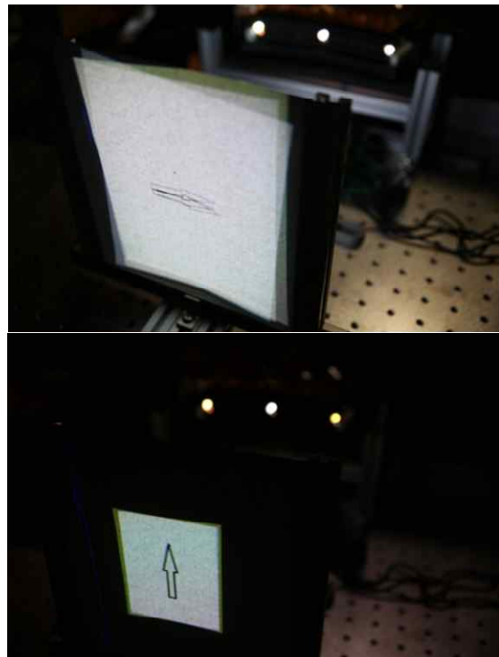
Figure 7. Experimental results before geometrical compensation (up) and after correction (down).
