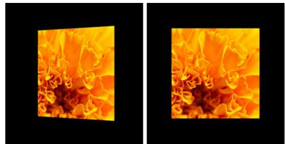
Figure 5. A distorted image from far right position (left) and compensated image by using homography matrix (right).
