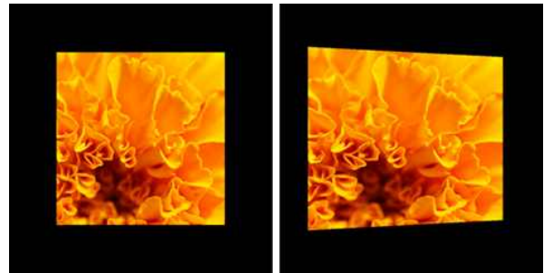
Figure 4. An original image of the projection optical module (left) and distorted image due to the toed-in geometry (right).
