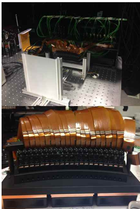
Figure 6. Experimental setup for verifying our compensation method (up) and enlarged image of toed-in configuration of disassembled projection optical modules (down).
