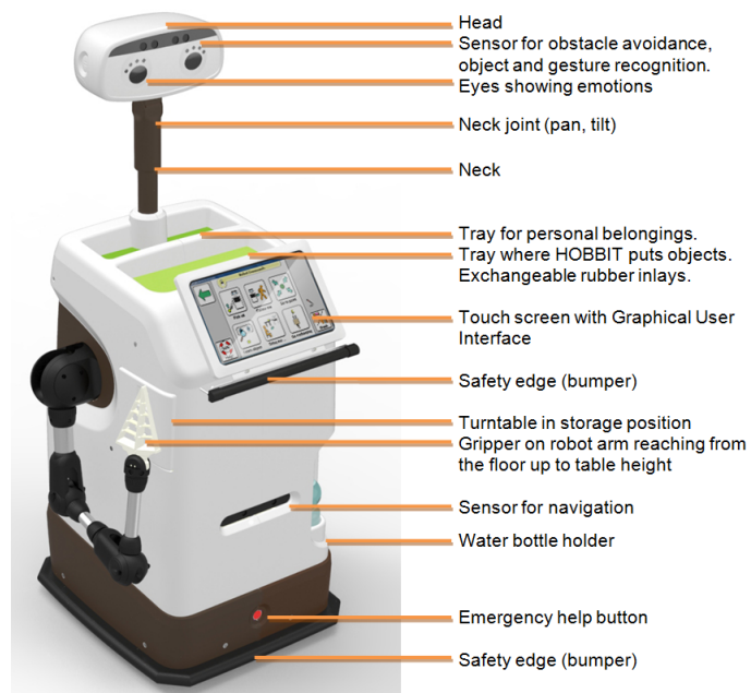
Figure 1. The Hobbit robot and its components.
