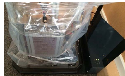
Figure 3. Docking station (black) and the robot wrapped in plastic for temperature tests.
