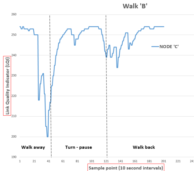
Figure 3. Walk 'B' LQI fluctuation for Node 'C'.
