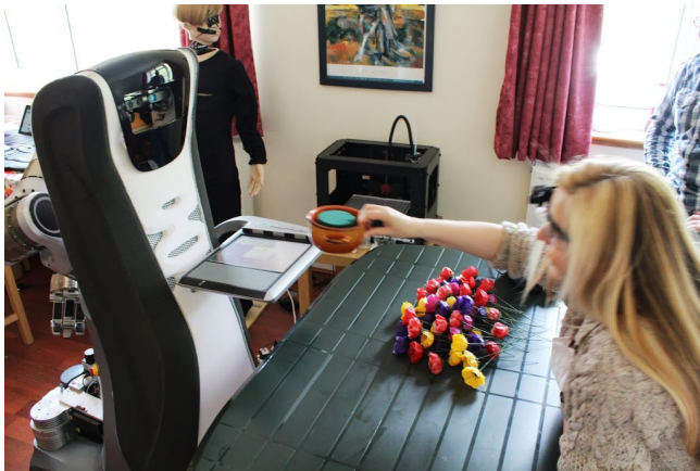
Figure 4. The University of Hertfordshire Robot House showing an HRI experiment with a Care-O-Bot 3 robot.
