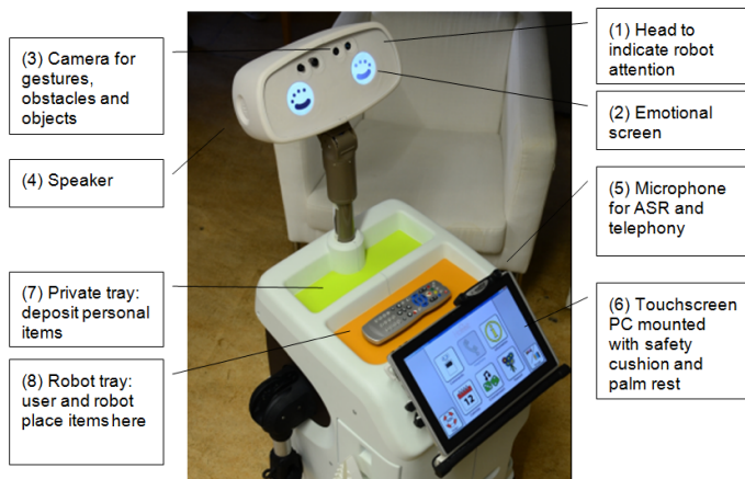
Figure 4. The upper body of Hobbit and its functionalities.
