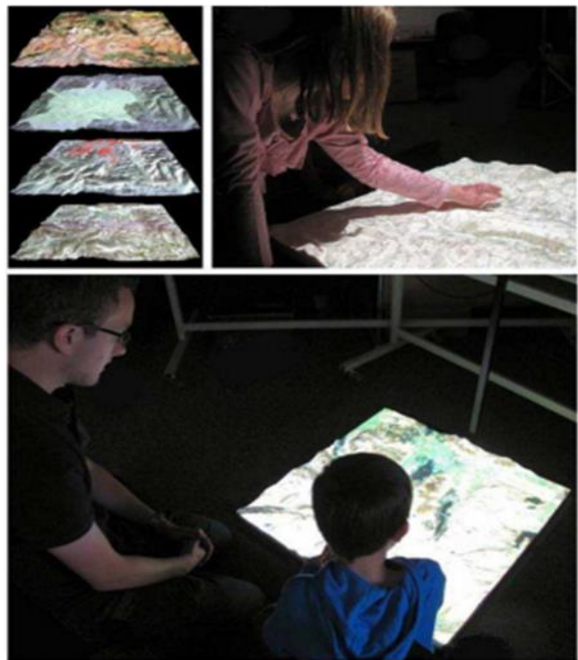
Figure 2: Projection Augmented Relief Model (PARM): Tangible Displays for Geographic Information. A selection of data layers used for projection (upper left); demonstrating at a community event at the University of Nottingham, 2011 (upper right and bottom) [8].
