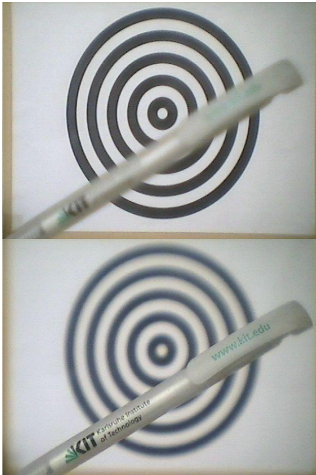
Figure 8. Active optical subsystem in operation. Top: adjustment mode for imaging of far distant objects. Bottom: adjustment mode for imaging of close objects.
