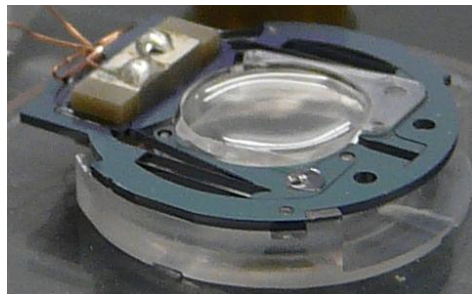
Figure 6. Varifocal optics assembled to the rear half shell of the glass housing.
