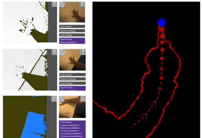
Figure 6: Distance between Kinect sensor and PARM, from top to bottom, 47 cm, 51 cm, 37 cm, shown variations in ability to detect fingertips. The coordinates of the finger as it approaches the model can be tracked and the last coordinate recorded before the finger merges with the model object is indicated in blue (right).
