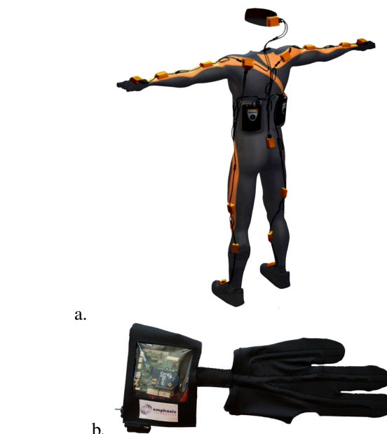
Figure 1. Wearable sensors used in the experiment: (a) XSens MVN suit [16]; (b) e-glove from Emphasis Telematics.
