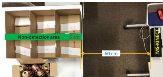
Figure 9. Experimental system for measuring delivery error rate
