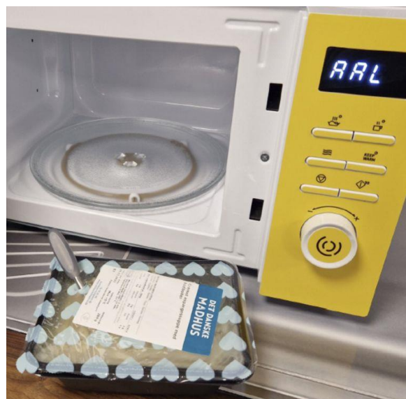
Figure 1. The adapted microwave and a meal with the probe inserted (Solution 1).
