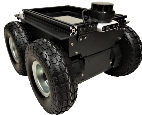
Figure 1. Teleoperated robotic system used in SLAM experiments.
