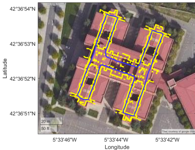
Figure 4. Map (yellow) and trajectory (blue) followed by the robot during the mapping of the Technological Building of the School of Industrial, Computer and Aerospace Engineering of the University of León.
