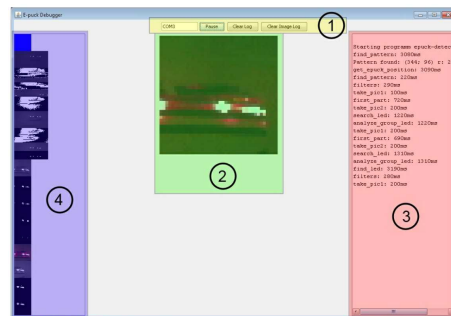
Figure 2. Developed software for monitoring the e-puck: (1) The required controls to establish the connection with the e-puck. (2) The real-time captured image. (3) Log statements (4) Archive of the last 20 captured pictures.
