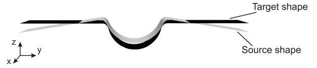
Fig. 1. Source and target shape of the hat profile.
