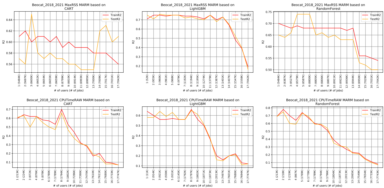
Fig. 4. R 2 Versus Number of Accounts in Predicting Memory and Time Using MARM Across Beocat
