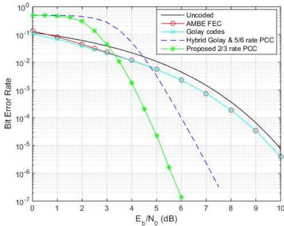
Figure 8. BER performance of uncoded, AMBE FEC, Golay (23,12) codes (AMBE FEC without scrambler), hybrid Golay (23,12) and 5/6 rate PCC and proposed 2/3 rate PCC.
