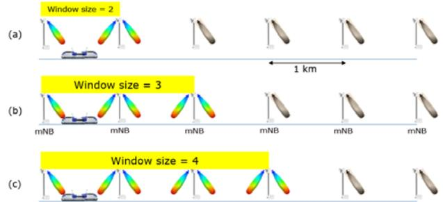
Figure 3. Assigned cases for window size. (a) Velocity is 100 km/hour as shown in subway. (b) Velocity is about 500 km/hour as shown in HST. (c) Velocity is about 750 km/hour for future HST.
