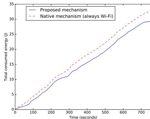
Figure 6. Comparison of the total consumed energy for both mechanisms for a 12-minute long segment of a download process.
