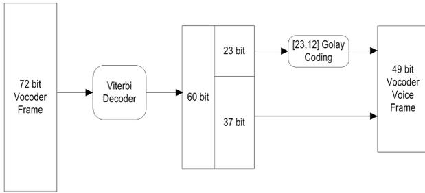
Figure 4. Hybrid FEC decoder block diagram for vocoder in [8].
