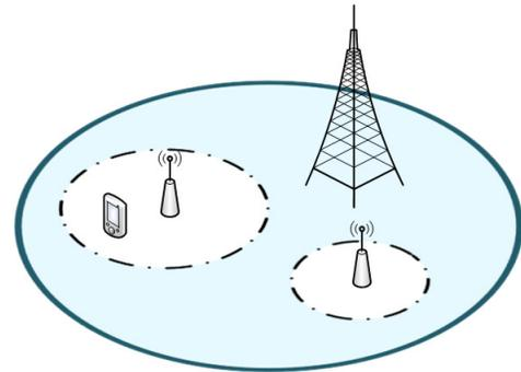
Figure 1. Representation of cellular and Wi-Fi network integration: full line circle – coverage area of a cellular network cell; dashed line circles – coverage areas of the Wi-Fi hot spots.
