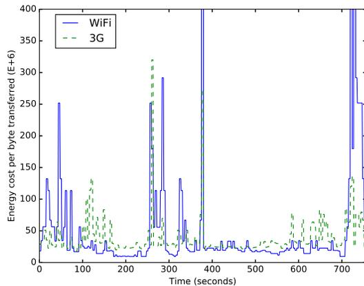
Figure 4. Energy cost per transferred byte for each network interface for a 12-minute long segment of a download process.
