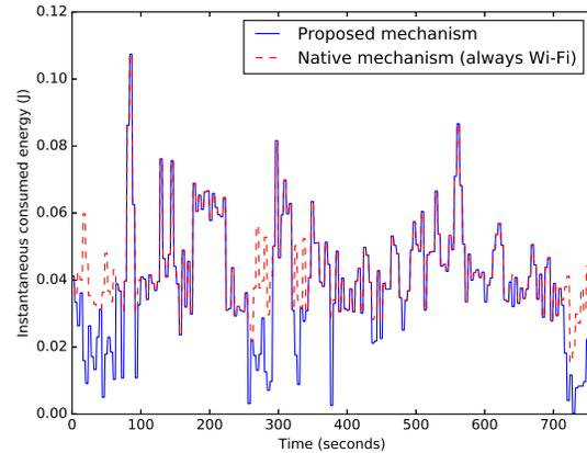
Figure 5. Comparison of the consumed instantaneous energy for both mechanisms for a 12-minute long segment of a download process.
