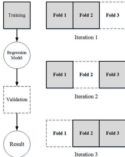
Figure 3. Diagram depicting the process of three-fold cross-validation. Adapted from [26].
