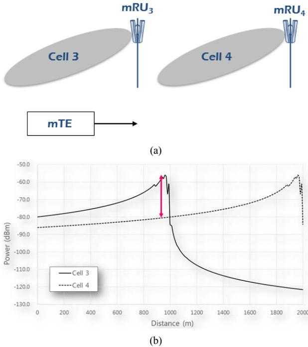
Figure 2. Cell search and time scheme for fast handover in MHN [13]. (a) Concept and (b) Scheme.
