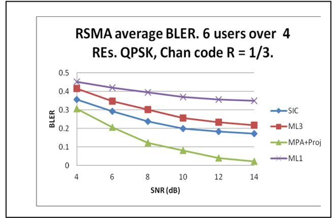
Figure 3. Simulation results for 6 users over 4REs. QPSK, Code Rate = 1/3.
