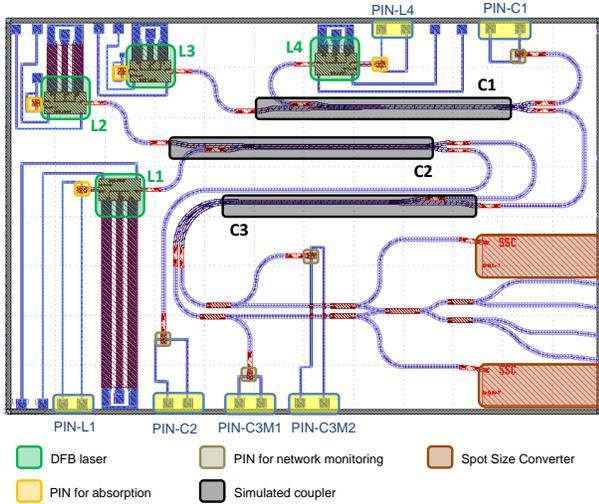
Figure 1. Design of an optical chip for data compression based on HT.
