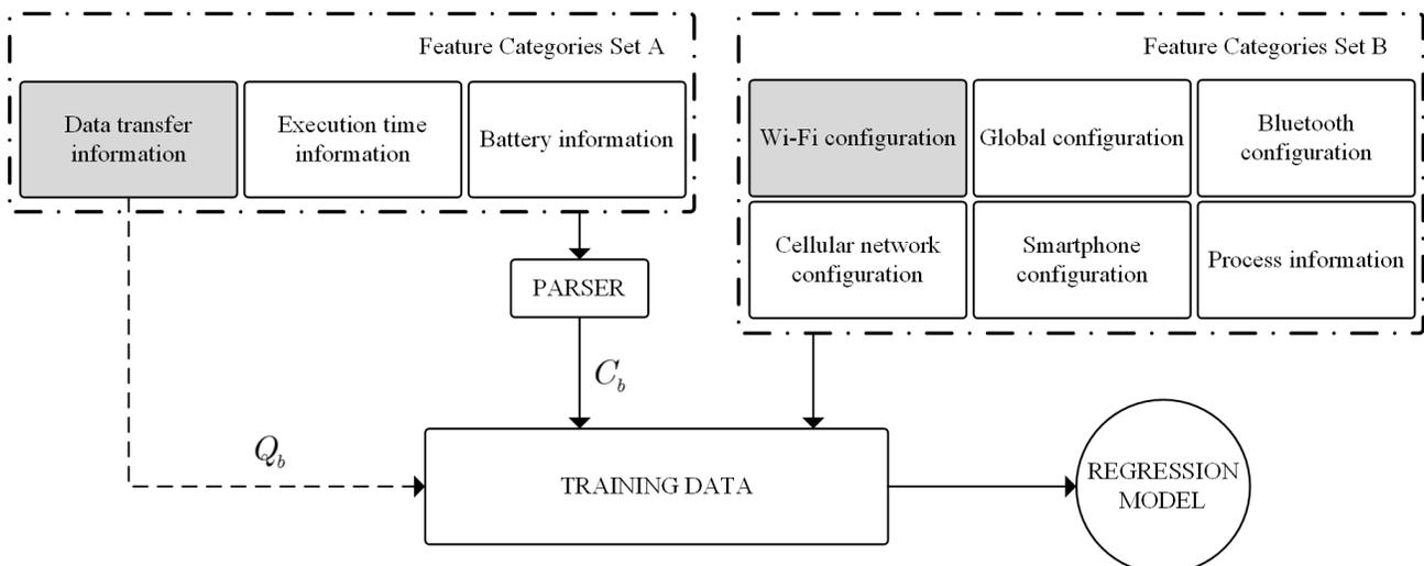
Figure 2. Diagram representing the creation of the regression model. The feature categories marked in grey are only used for the Wi-Fi models.
