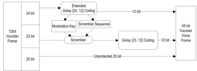
Figure 2. 3600 bps AMBE's vocoder FEC decoder scheme.
