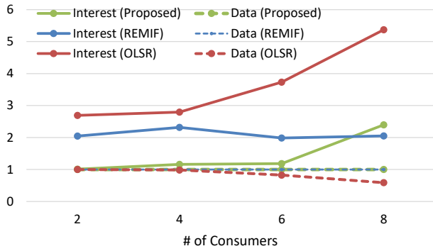
Figure 8. Numbers of Interest packets actually sent from consumers and Data packets received by consumers (normalized by originated Interests; consumers requesting same content).
