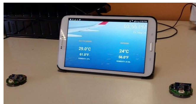
Figure 3. Main Interface of the BLE-based android application for acquiring environmental data.
