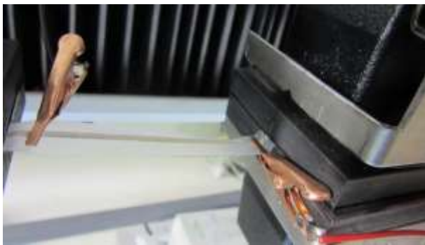
Figure 1. Conductivity test on a stretchable substrate during a contract and relax process.
