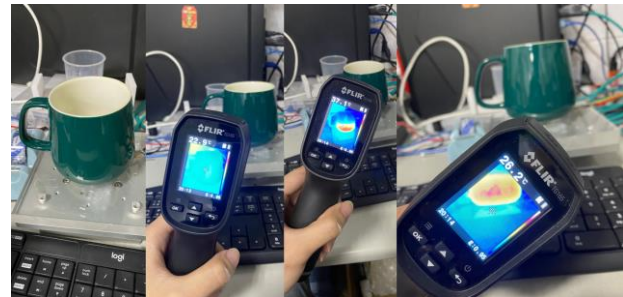
Figure 14. Infrared thermal imager temperature change
