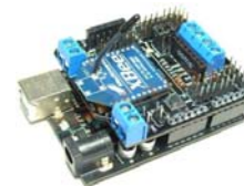
Figure 7. The control board with an xBee-shield attached.
