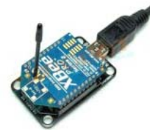
Figure 6. The xBee wireless component serving as the coordinator.
